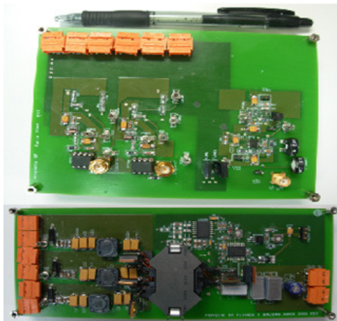
Fig. 11. Photograph of implemented multilevel converter, architecture two.
