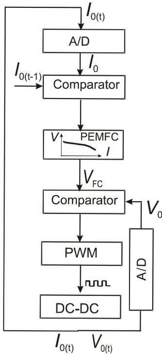
Fig. 4. Block diagram of the control algorithm.
