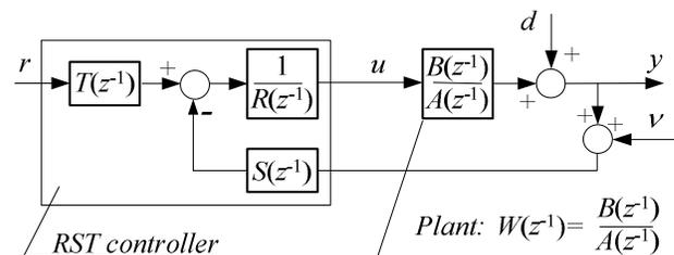
Fig.1 RST control structure.
