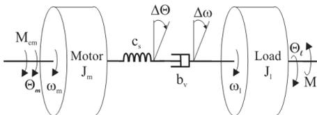
Fig. 2. Flexible coupling of motor axle and load.
