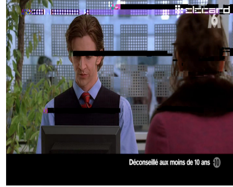
Fig. 3. Video frame degraded by packet-loss.
