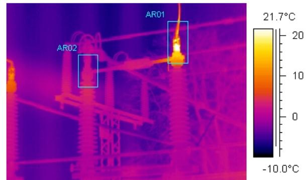
Figure 6. Thermogram of the busbar disconnector F4 in TL 110 kV Goražde 2 in the FU 110/35/20/10 kV Goražde 1
