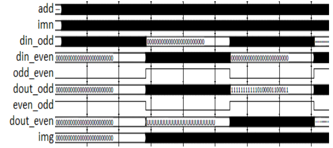
Fig. 16. Timing diagram of first Image accumulation process.
